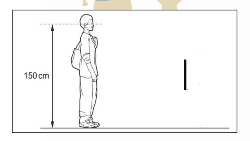
The distance between the top of the mirror and the ground is 75cm
